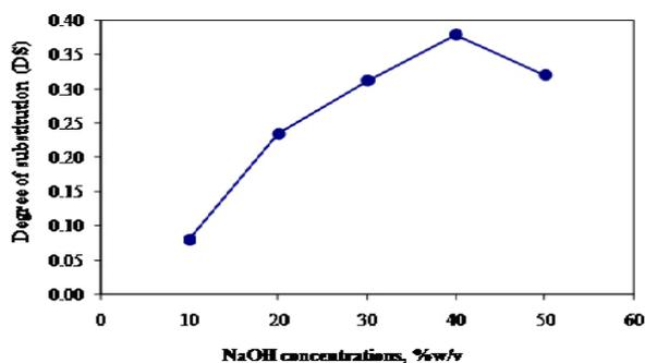
Figure 3. Effect of various NaOH concentrations on DS of CMS<sub>r</sub>
