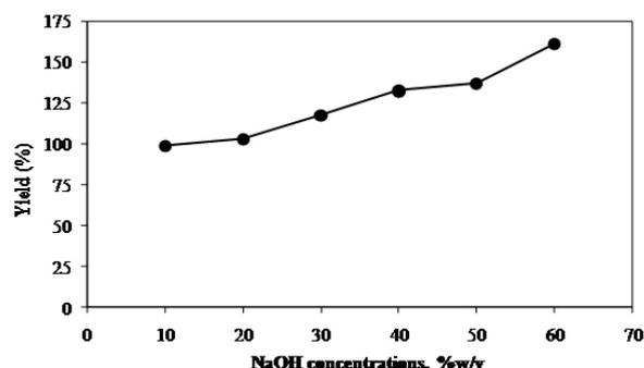
Figure 1. Percent yield of carboxymethyl rice starch synthesized with various NaOH concentrations (10, 20, 30, 40, 50 and 60 %w/v)
