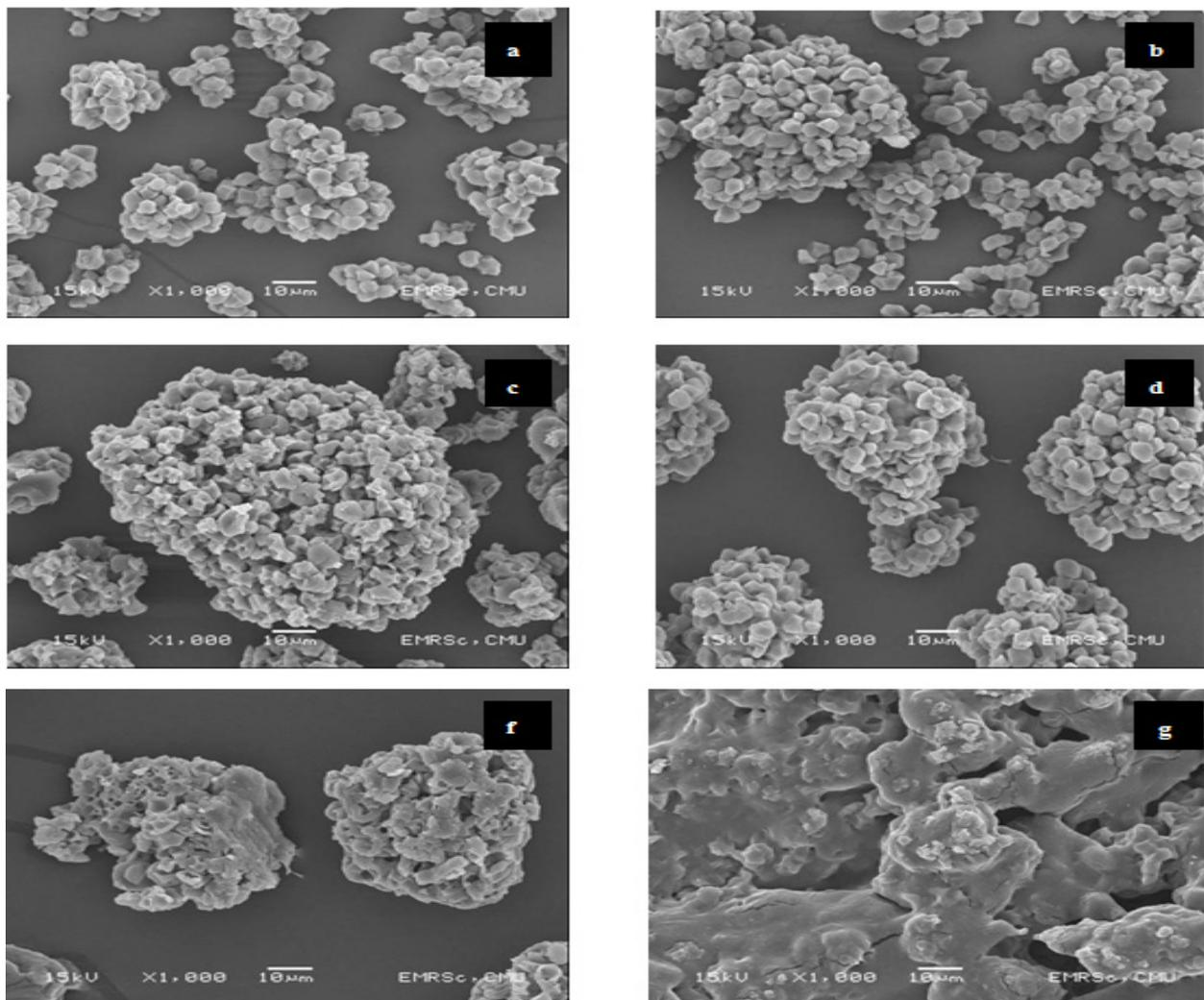
**Figure 4.** Scanning electron micrographs of a) native rice starch and CMS<sub>r</sub> synthesized with NaOH concentrations at b) 10%, c) 20%, d) 30%, e) 40%, f) 50% and g) 60%: 1000x
