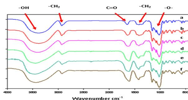
Figure 2. Infrared spectrum of a) native rice starch, CMS<sub>r</sub> synthesized with various NaOH concentrations at b) 10%, c) 20%, d) 30%, e) 40% and f) 50%
